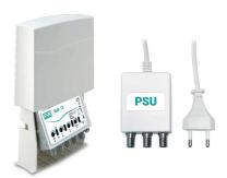
1-input (III+DAB+UHF) mast amplifier with 42dB gain and up to 116dB $\mu$ V output level on UHF band, separate VHF/UHF amplification with independent gain adjustment (0-15dB) for each band and low noise figure. T2 technology with UHF cut band for LTE 4G @790MHz and 5G @694MHz.
